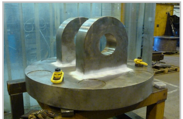
Top: 100mm thick eye beams positioned into re-machined slots ready for welding
